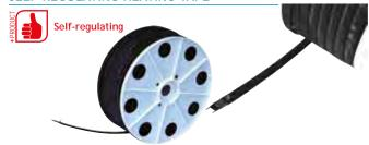
Heating tape protects against freezing and avoids the deterioration of metal water supply pipes. It is made with two conducting wires surrounded by an insulating material containing conductive graphite.
