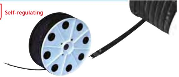
Heating tape protects against freezing and avoids the deterioration of metal water supply pipes. It is made with two conducting wires surrounded by an insulating material containing conductive graphite.
