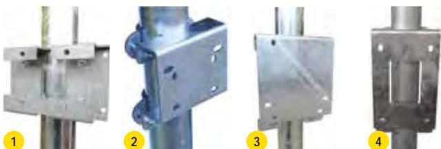
The mounting plate is used to fasten the drinker with the metallic protection on round Ø 76 or 102 mm posts using its two 1/2 toothed flanged for an anti-rotation point. It is designed with technical reinforcements and screw holes. Delivered with one pair of 1/2 round flanges.
