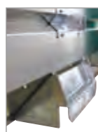
3-point hitch. Reinforced by a thick bolted plate.
